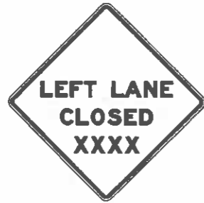
LEFT LANE CLOSED SIGN
